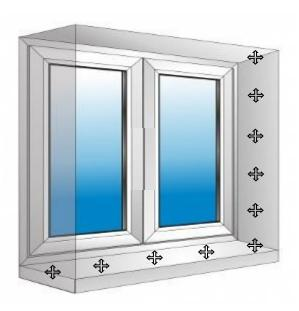
**STEP 2**: Put the wall plugs into the holes and screw the anchors
